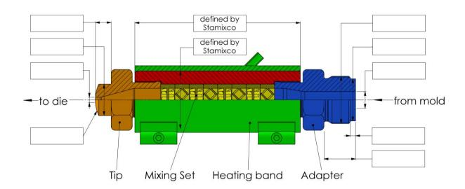
Standard Thickness of Heating band: 3.5mm-7mm depending on operating temperature
