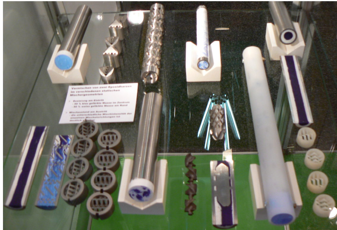
Top row: ISG Type „House“ Design Empty Pipe Bottom row: X-Type with ring 3-Blade Helical Pineapple XPS
