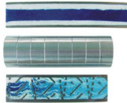
Mixing of epoxy resins in an empty pipe and in an mixer LMXR
