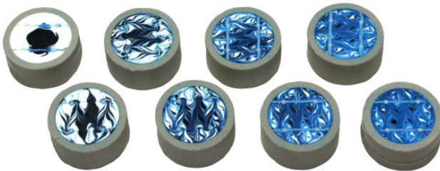
Static Mixer SMB-GXS – DN40 Mixing efficiency through SMB-GXS with white and blue epoxy resins
